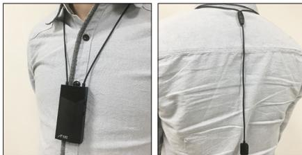
\* Note: Fix your AM-600 to the target person or object properly. For better tracking effect, wear a positioner with the smooth and transparent side facing out.
