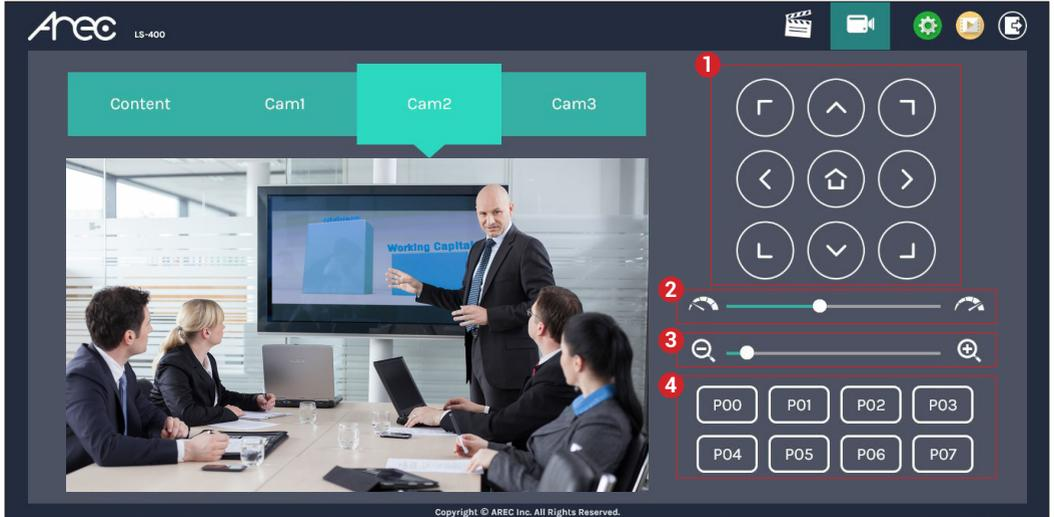
1. Direction control panel: Click the arrow buttons to move the camera.
